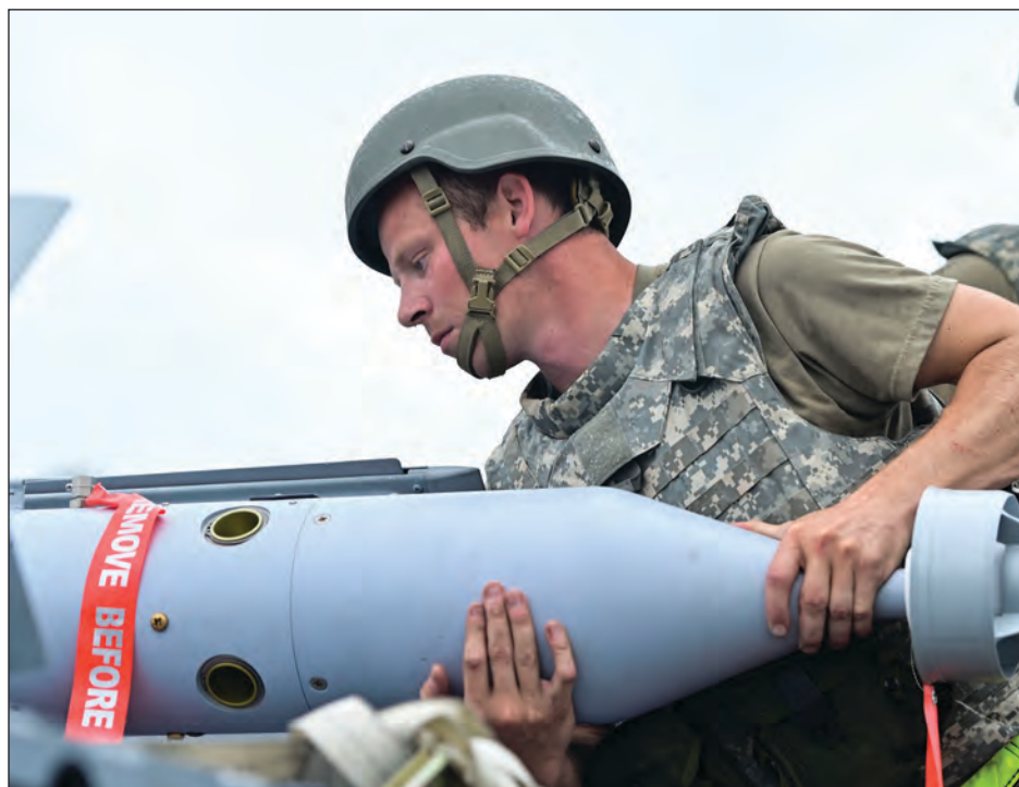
U.S. Air Force Senior Airman Keaton Hartsook, 20th Equipment Maintenance Squadron conventional maintenance crew chief, attaches the MAU-169 computer control group to the GBU-12 bomb during Iron Hand 24-03 at North Auxiliary Airfield. The 20th EMS built a total of 240 sticks of chaff and flare and nine bombs at the contingency location.
