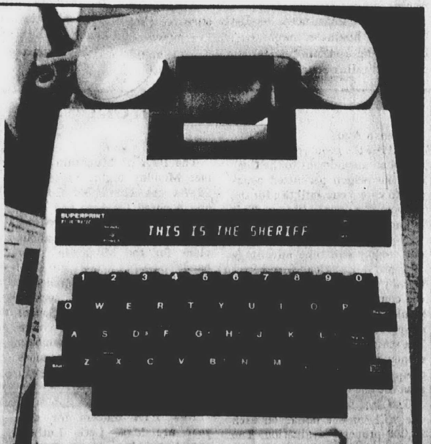
device is operated by typing a message which is transmitted to a receiver and displayed on a screen. Sherry Hillburn with the Arkansas Department of Health and Human Services said assistance in obtaining one of the TDD units is available through several sources.
